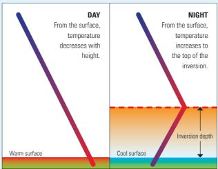
Above: Typical vertical temperature profiles for a point in time during the night and day. The day profile typically cools with height and the night profile typically warms with height to a depth which constitutes the surface temperature inversion layer. The point where the temperature stops increasing is the top of the surface temperature inversion layer.
